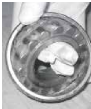
Fig. 21. Grease can easily be packed by hand.
