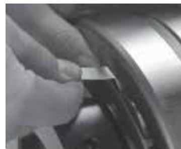
Fig. 18. Measure RIC before installation.
